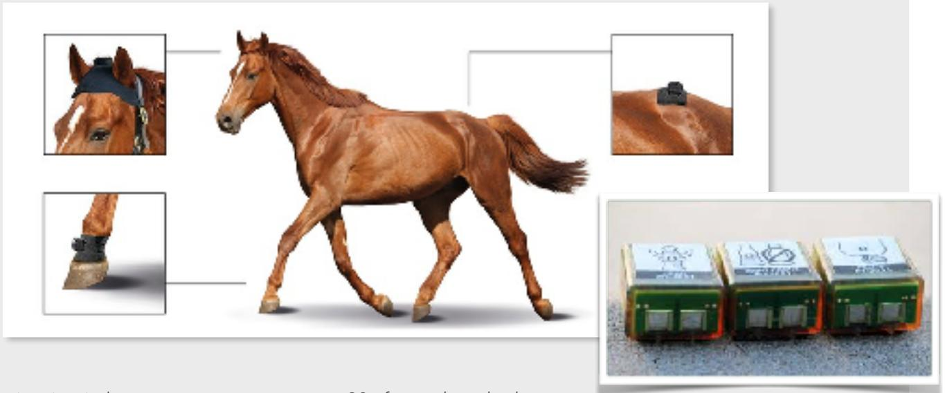
Equinosis wireless sensors measure up to 20x faster than the human eye, tracking movement accurately to within millimetres, making the system accurate, sensitive and precise - something hugely helpful and necessary when assessing multi-limb lameness and low grade lameness and performance issues.
