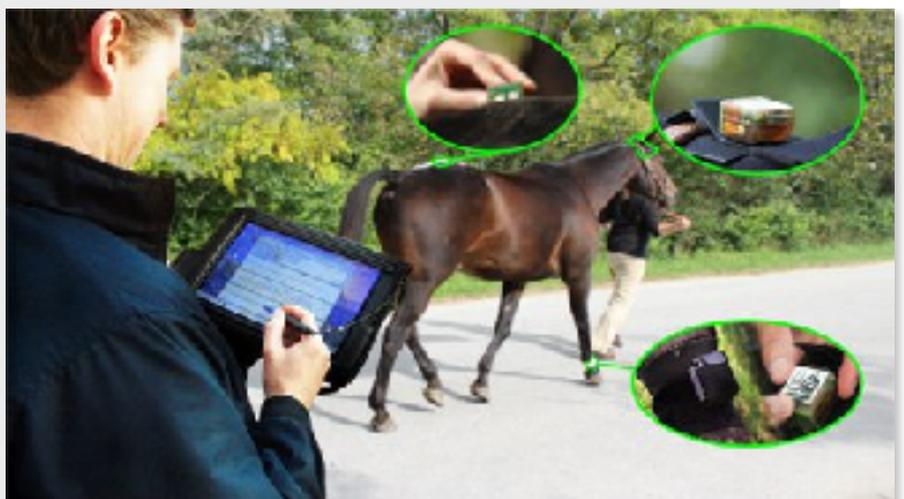
from many years of research, which utilised treadmills and high-speed cameras to mathematically characterise normal and impaired gait, measuring vertical acceleration of the torso to determine asymmetries in head and pelvic position between left and right halves of stride at the University of Missouri. Translational research then adapted the analysis to be used as a convenient, robust, miniaturised system in the field.
